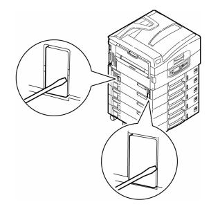
3. Install the metal brackets where the breakout panels were.
